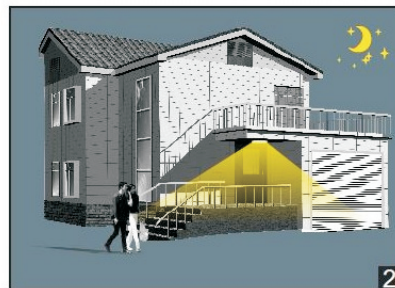
2 With insufficient daylight,even when motion detected.light ON.
